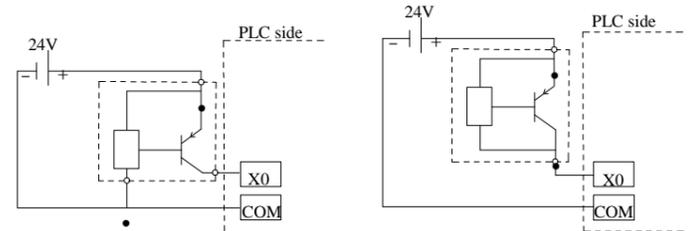
3-wire (PNP) proximity switch wiring 2-wire (PNP) proximity switch wiring
