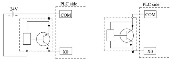
3-wire (NPN) proximity switch wiring 2-wire (NPN) proximity switch wiring
