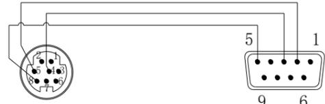
Mini Din 8-core plug (pin)
