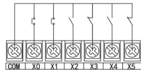
Switch button wiring
